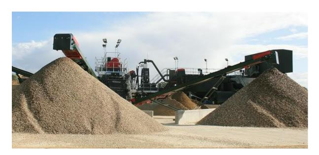
Above is the Recycling Plant which produces many recycled products including Clay, Washed 0/2 FP and 0.4 MP Concrete san as well as 2/10, 10/20, 20/40 single size recycled products. Also produced on mobile plants (not pictured) are 6F5, Crushed Concrete Type 1, Asphalt Planning and Screened soils.
